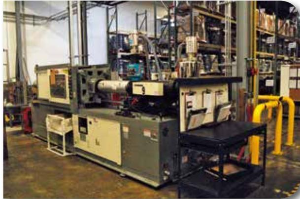
Injection molding machine for prototyping and short production runs.
