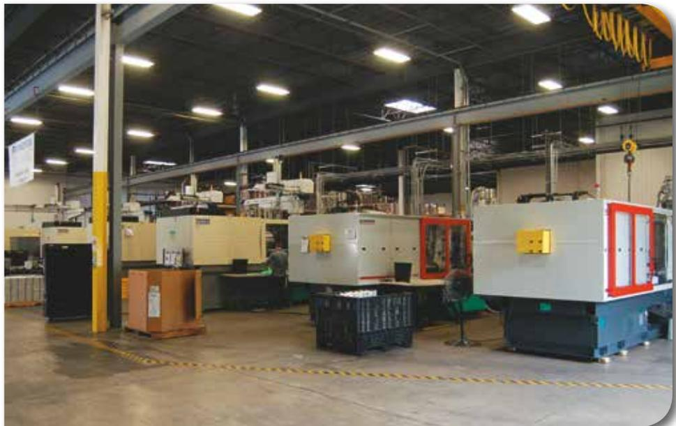
State-of-the-art, high capacity, injection molding machines.
