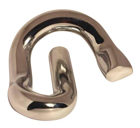
The 'e' series clip with its unique geometric design offers a lightweight, low cost rail fastening. Spring and torsion work together to provide a high clamping force, excellent resistance to rail rollover and longitudinal restraint.
